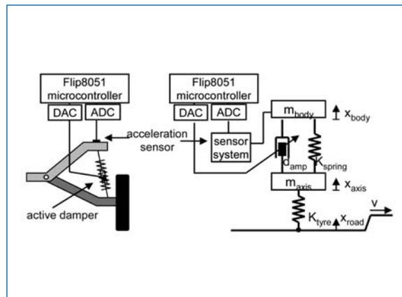
Figure 1. Active car suspension
