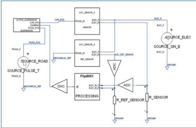
Figure 2. Modeling of a semi-active car wheel suspension
