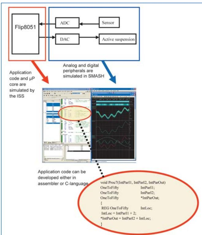
Figure 3. Debugging and simulation/validation possibilities of the embedded software in the system environment
