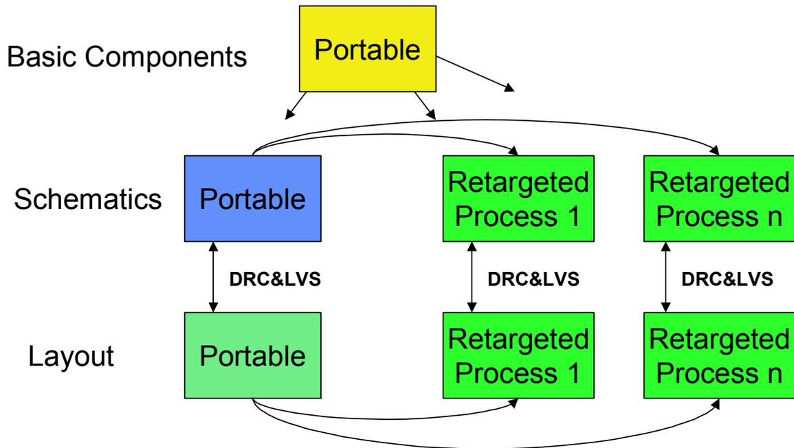
This methodology for portable design rules and powerful verification system allows to save a lot of time on several ways:
