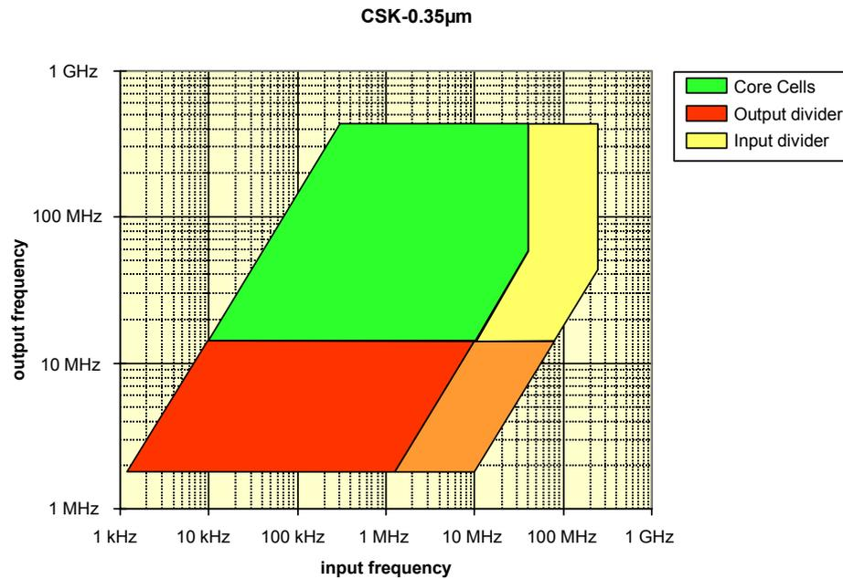
A typical extension of the working area is shown on the slide.
