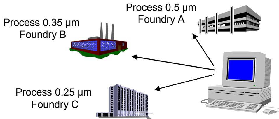
Retargeting = migration of schematics and layout designed with portable rules towards a targeted process
