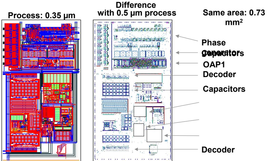
To illustrate what has been said on the retargeting methodology test circuits of the generator ADMIR has been successfully fabricated for three technological processes, one 0.5  $\mu\text{m}$  process and two 0.35  $\mu\text{m}$  processes.
