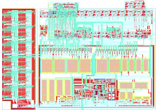
The result of the generator for the second example of flexible ADC is shown on the slide. The complexity for the analog and logic parts are lower than the previous example. This cut has also been implemented in a 0.35 μm pure logic CMOS process, the silicon are of the analog section was 0.3 mm<sup>2</sup> and the power consumption less than 1.3 mA.
